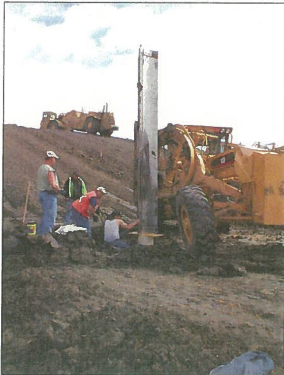
8 - Pressing large block sample ring with Cat motor grader on 1.0E-7 test fill
