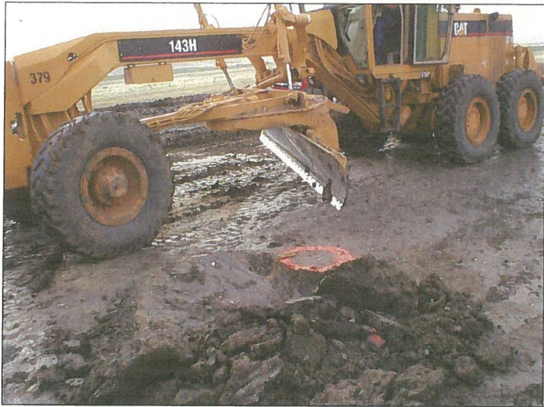
7 - Cutting around 1.0E-7 (west side) large block sample with Cat motor grader
