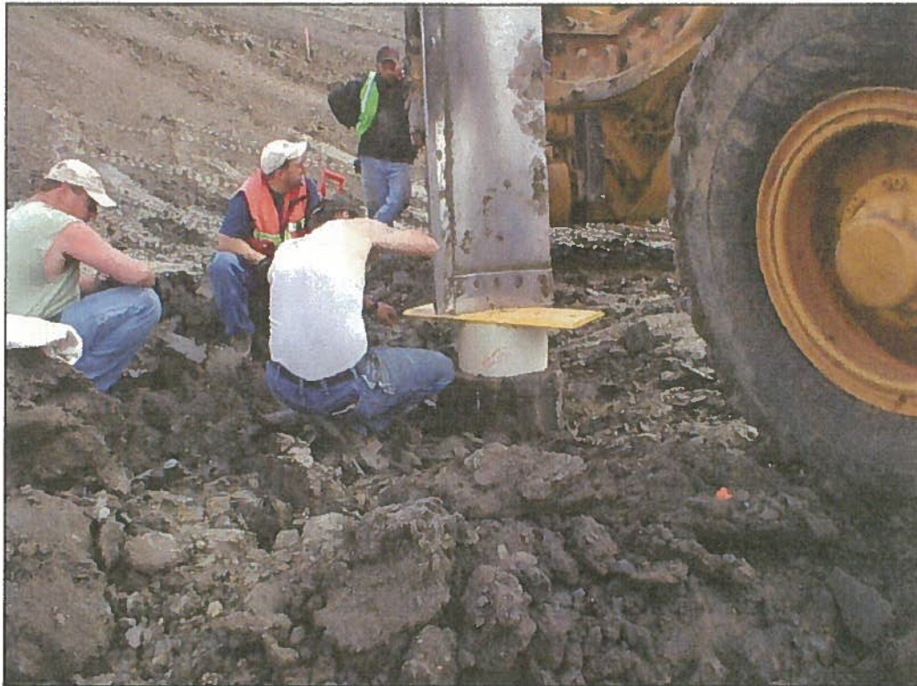
9 - Pressing large block sample ring with Cat motor grader on 1.0E-7 test fill
